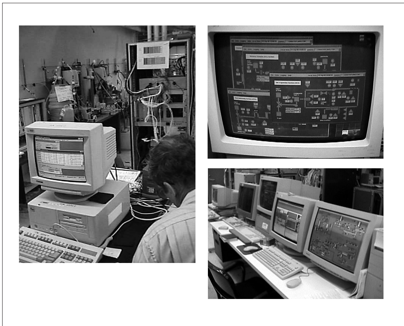
Figure 6. 3T Control Computers for the INTEGRATED WATER-RECOVERY SYSTEM.
